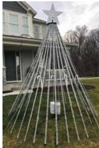
360 MegaTree Kit - 32 Strands of 50 Bullet Pixels. - Kit purchased from holidaycoro. - Star topper purchased from Boscoyo.
